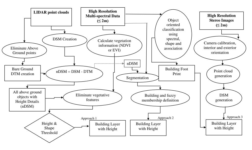
Figure 4: Building Extraction Process from Remote Sensing Data
