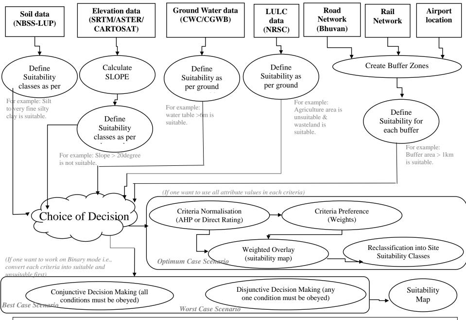
**Figure 6: Solid Waste Disposal Site Suitability Modelling using RS & GIS.** (NBSSLUP – National Bureau of Soil Survey and Land Use Planning; CWC – Central Water Commission; CGWB – Central Ground Water Board; NRSC – National Remote Sensing Centre).
